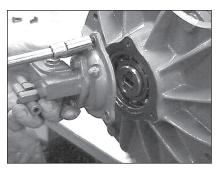
2. Remove the 3 6x20mm screws attaching the oil pump assembly to the vacuum pump.
