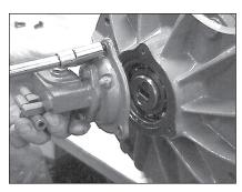
Reinstall the oil pump drive key, oil pump mount assembly, and gaskets to the pump.
