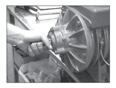
15. At this point you should be able to turn the pump by hand.
