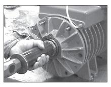
12. Lubricate seal sleeve and install the endplate on the end of the rotor and carefully drive the endplate on the rotor.
