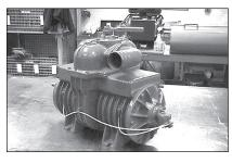
24. Start the pump at a slow RPM and allow to run for a few minutes until oil can be seen in the lines or dripper.
