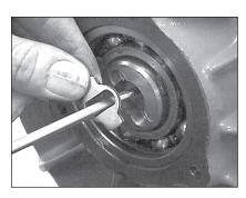
3. Remove the oil pump drive key from the end of the rotor.
