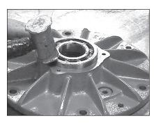
9. Lubricate and install the bearings in the endplates.
