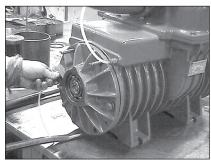
18. When the endplate is close enough to the housing install the endplate bolts lift the endplate-rotor assembly to allow proper alignment of the bolts and bolt holes and start the bolts into the housing.
