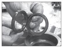
8. Locate the replacement seals and install them in the endplates with the seals positioned back to back.
