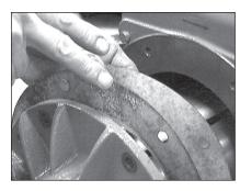
11. Locate the proper number of gaskets and install them on the endplate.
