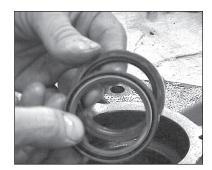
6. Inspect vanes, bearings and seals and replace as necessary.
