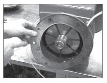
5. Note the number of gaskets on the endplate. You must use the same number of gaskets during reassembly.
