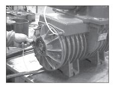
13. When the endplate is close enough to the housing install the endplate bolts lift the endplate-rotor assembly to allow proper alignment of the bolts and bolt holes and start the bolts into the housing.
