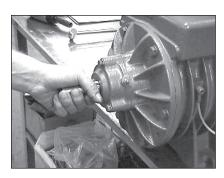
22. Lubricate and reinstall the front outboard bearing and bearing cover.
